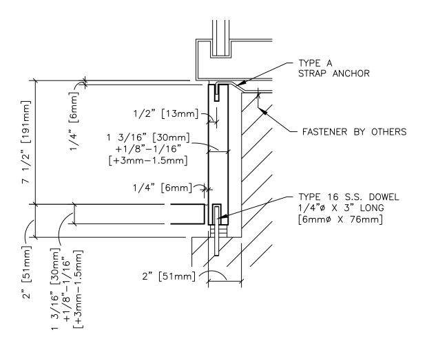
BASE DETAIL - ANCHOR AT TOP AND BOTTOM
