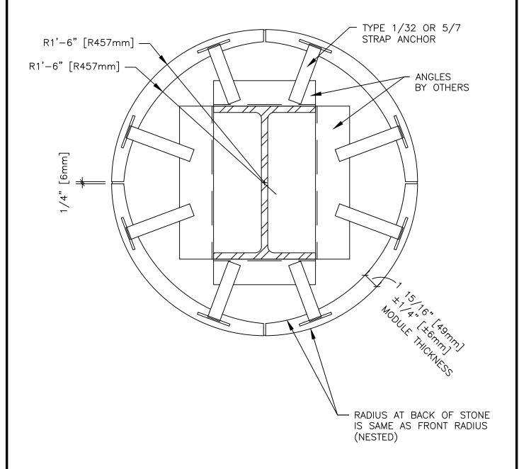
PLAN — COLUMN COVER RADIAL NESTED BEAM & ANGLE BACKUP
