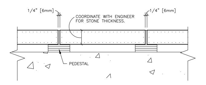
PAVING JOINT PEDESTAL SECTION
